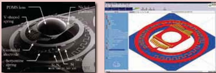
Electrostatic actuated micro-lens for biomedical application (With courtesy of University of British of Columbia and British Columbia Cancer Research Centre, CANADA)
